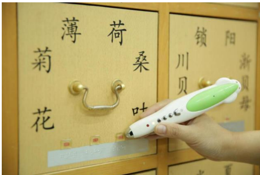
Figure 3. Diagram of the Voice QR Code Reading pen on the medicine cabinet [18]
